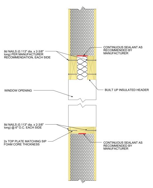
ALL SIP JOINTS SHALL BE AIR SEALED WITH SEALANT AND/OR SIP TAPE. FOLLOW SIP MANUFACTURER'S RECOMMENDATIONS FOR SIP TAPE WIDTHS AND SEALANT PATTERN AND THICKNESSES.
