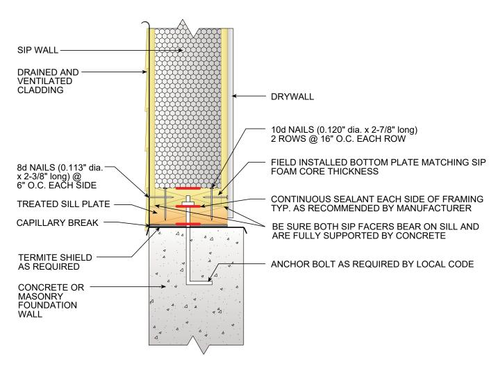
ALL SIP JOINTS SHALL BE AIR SEALED WITH SEALANT AND/OR SIP TAPE. FOLLOW SIP MANUFACTURER'S RECOMMENDATIONS FOR SIP TAPE WIDTHS AND SEALANT PATTERN AND THICKNESSES.
