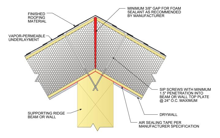
ALL SIP JOINTS SHALL BE AIR SEALED WITH SEALANT AND/OR SIP TAPE. FOLLOW SIP MANUFACTURER'S RECOMMENDATIONS FOR SIP TAPE WIDTHS AND SEALANT PATTERN AND THICKNESSES.
