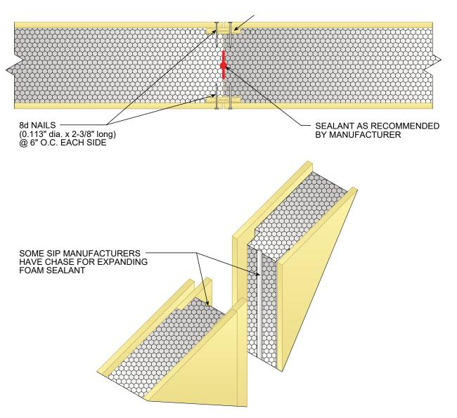
ALL SIP JOINTS SHALL BE AIR SEALED WITH SEALANT AND/OR SIP TAPE. FOLLOW SIP MANUFACTURER'S RECOMMENDATIONS FOR SIP TAPE WIDTHS AND SEALANT PATTERN AND THICKNESSES.
