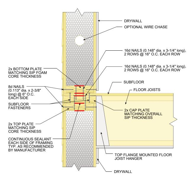
ALL SIP JOINTS SHALL BE AIR SEALED WITH SEALANT AND/OR SIP TAPE. FOLLOW SIP MANUFACTURER'S RECOMMENDATIONS FOR SIP TAPE WIDTHS AND SEALANT PATTERN AND THICKNESSES.
