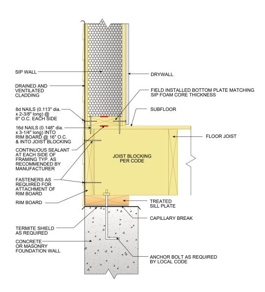
ALL SIP JOINTS SHALL BE AIR SEALED WITH SEALANT AND/OR SIP TAPE. FOLLOW SIP MANUFACTURER'S RECOMMENDATIONS FOR SIP TAPE WIDTHS AND SEALANT PATTERN AND THICKNESSES.
