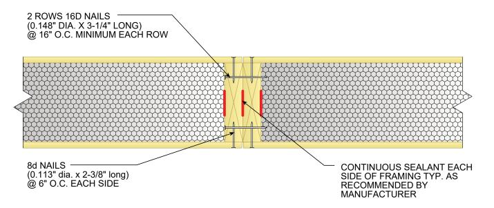
ALL SIP JOINTS SHALL BE AIR SEALED WITH SEALANT AND/OR SIP TAPE. FOLLOW SIP MANUFACTURER'S RECOMMENDATIONS FOR SIP TAPE WIDTHS AND SEALANT PATTERN AND THICKNESSES.
