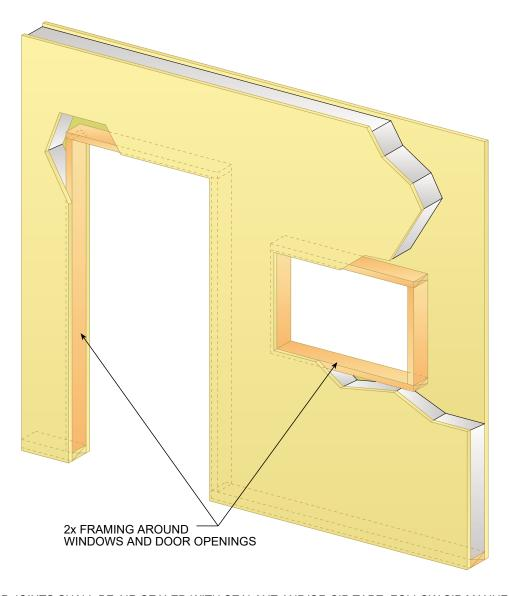
ALL SIP JOINTS SHALL BE AIR SEALED WITH SEALANT AND/OR SIP TAPE. FOLLOW SIP MANUFACTURER'S RECOMMENDATIONS FOR SIP TAPE WIDTHS AND SEALANT PATTERN AND THICKNESSES.
