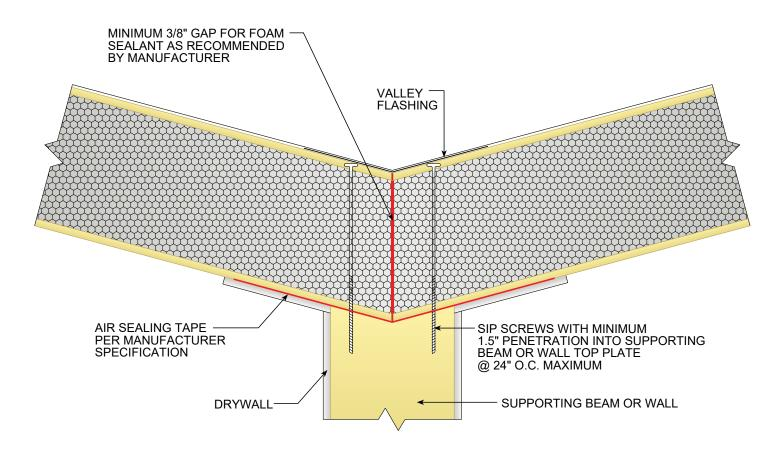
ALL SIP JOINTS SHALL BE AIR SEALED WITH SEALANT AND/OR SIP TAPE. FOLLOW SIP MANUFACTURER'S RECOMMENDATIONS FOR SIP TAPE WIDTHS AND SEALANT PATTERN AND THICKNESSES.
