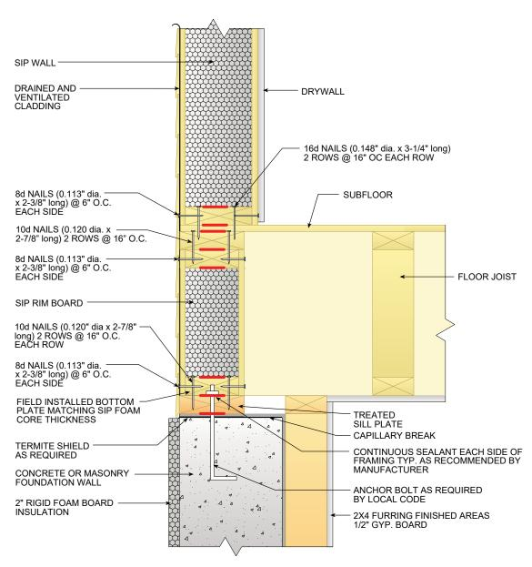
ALL SIP JOINTS SHALL BE AIR SEALED WITH SEALANT AND/OR SIP TAPE. FOLLOW SIP MANUFACTURER'S RECOMMENDATIONS FOR SIP TAPE WIDTHS AND SEALANT PATTERN AND THICKNESSES.
