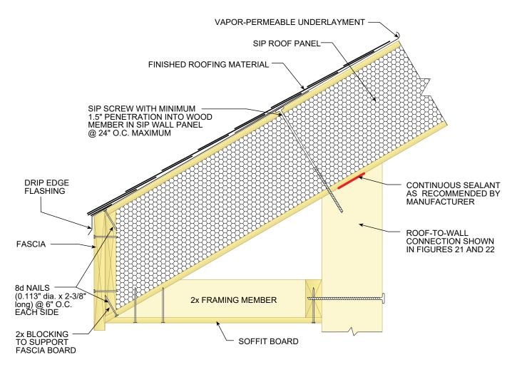
ALL SIP JOINTS SHALL BE AIR SEALED WITH SEALANT AND/OR SIP TAPE. FOLLOW SIP MANUFACTURER'S RECOMMENDATIONS FOR SIP TAPE WIDTHS AND SEALANT PATTERN AND THICKNESSES.
