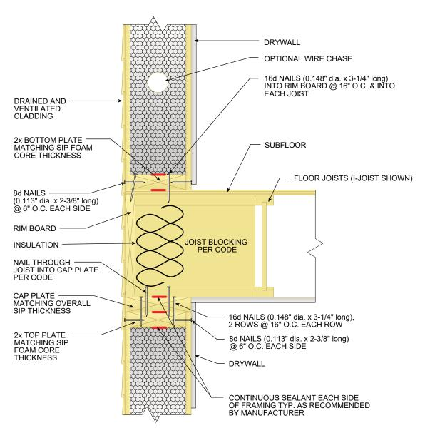
ALL SIP JOINTS SHALL BE AIR SEALED WITH SEALANT AND/OR SIP TAPE. FOLLOW SIP MANUFACTURER'S RECOMMENDATIONS FOR SIP TAPE WIDTHS AND SEALANT PATTERN AND THICKNESSES.
