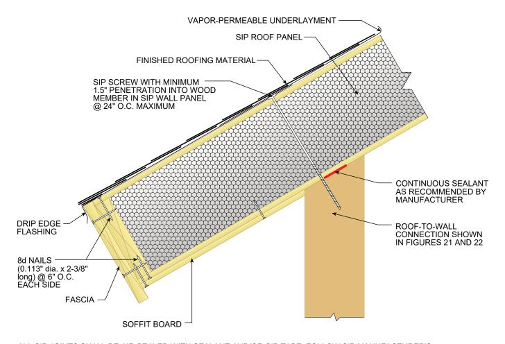
ALL SIP JOINTS SHALL BE AIR SEALED WITH SEALANT AND/OR SIP TAPE. FOLLOW SIP MANUFACTURER'S RECOMMENDATIONS FOR SIP TAPE WIDTHS AND SEALANT PATTERN AND THICKNESSES.
