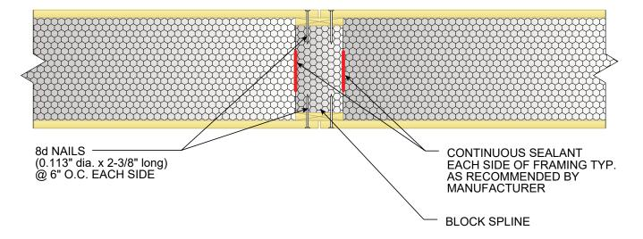
ALL SIP JOINTS SHALL BE AIR SEALED WITH SEALANT AND/OR SIP TAPE. FOLLOW SIP MANUFACTURER'S RECOMMENDATIONS FOR SIP TAPE WIDTHS AND SEALANT PATTERN AND THICKNESSES.
